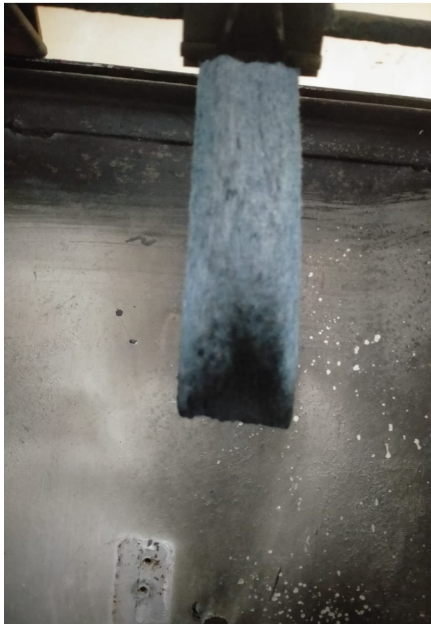
Fig.1: Fire not burn up to holding clamp during Fire Retardant Test.
